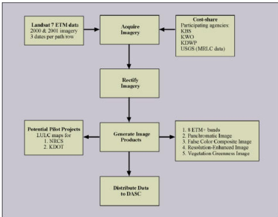
**Figure 1.** A flowchart illustrating the methodology of developing the Landsat 7 Imagery Database for Kansas.
