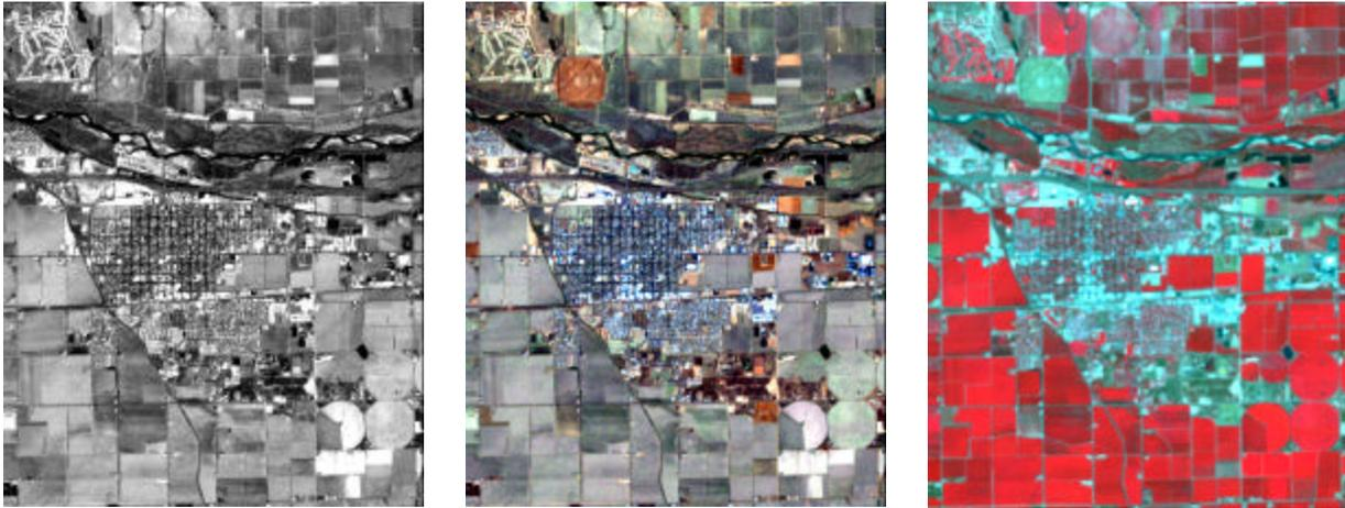
**Figure 2a.** The panchromatic band with 15m spatial resolution, **2b.** A resolution-enhanced natural color composite (pan merged with multispectral bands 3, 2, and 1), **2c.** A false-color composite (bands 4, 3, and 2).
