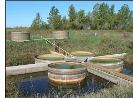
80 tank mesocosms 7.3 m 2 , 10 m 3 and 1.5 m deep, filled in groups in the same manner as the ponds
