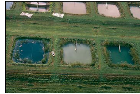
77 pond mesocosms, 0.045 ha, 450 m 3 and 2.7 m deep with natural clay bottoms, filled in groups with natural pond water and biota to begin an experiment
